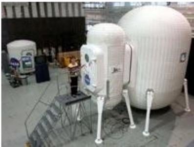
*NASA's Exploration Technology Development Program is working on designs for a Moon habitat. The light-weight experimental house shown here is inflatable, so would not take up much*
